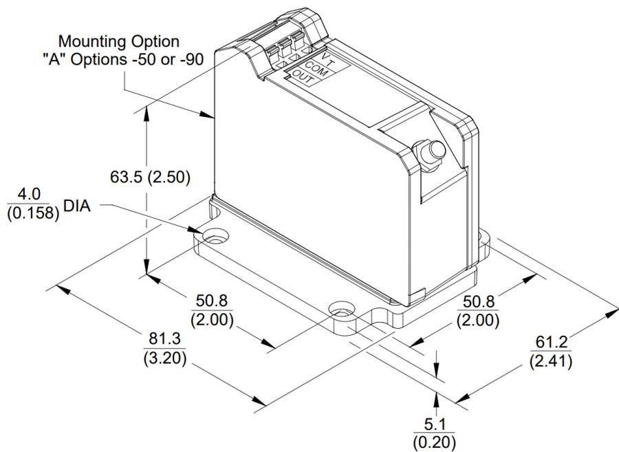
**Figure 18: 330850 Panel Mount 3300 XL 25mm Proximitor Sensor**
