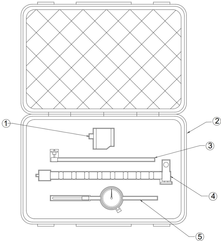
**Figure 22: 163854 Dial Indicator Verification Kit (with cover open)**
