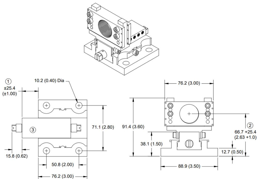
**Figure 20: 330853 Sliding Bracket, Single DE Version**
