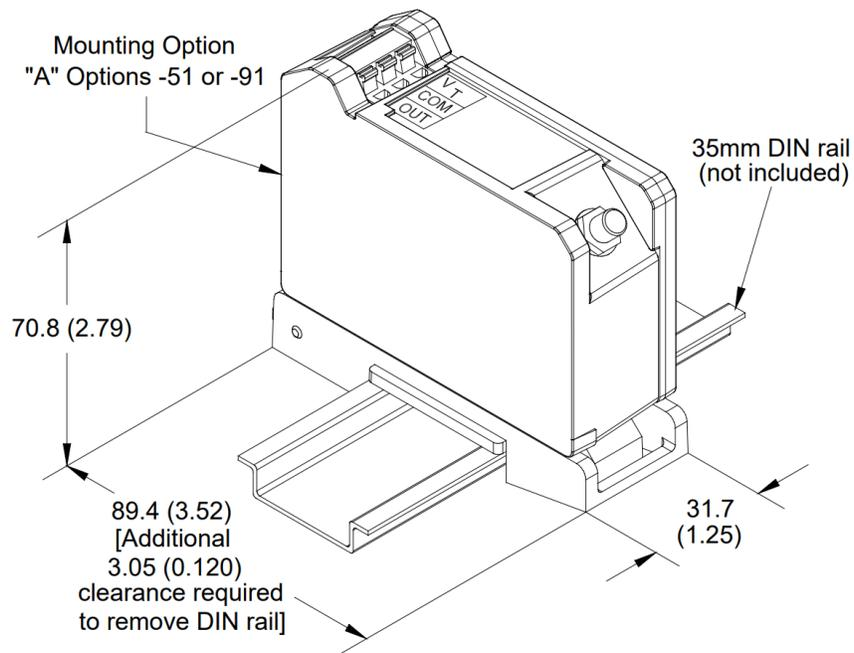
**Figure 19: 330850 DIN Mount 3300 XL 25mm Proximity Sensor**
